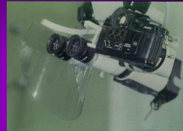
1. **Beam coaxial with microscopic viewing** and aiming beam visible through the optical lenses controlled with a joystick, distance 200-400 mm, magnif. power 6-40 X.
