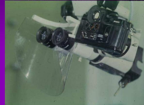
1. **Beam coaxial with microscopic viewing** and aiming beam visible through the optical lenses controlled with a **joystick**, distance 200-400 mm, magnif. power **6-40 X**.
